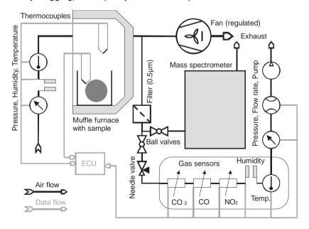
Fig. 2. Schematic of the laboratory fire simulator
