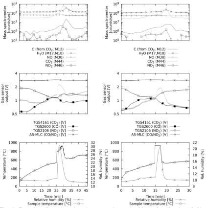
Fig. 6. Results of two combustion experiments with hydraulic pipe (left) and corrugated hose (right).
