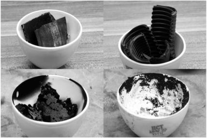
Fig. 4. Two samples before (top) and after (bottom) combustion. (Left) Hydraulic pipe from a truck, fiber enforced elastomer. (Right) Corrugated hose from a passenger car's cable harness, polyamide-6.
