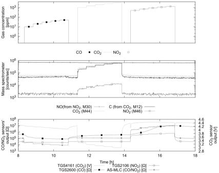
Fig. 5. An example of the measurements done under lab conditions using a gas mixing system and pure gases. Both the results of the mass spectrometer (mid) and the gas sensor array (bottom) are shown.
